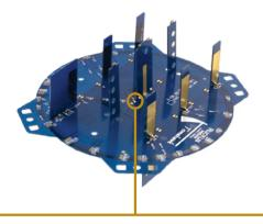
A patented smart antenna array integrates six high-gain vertically and horizontally-polarized antenna elements. With BeamFlex, this enables up to 4096 potential antenna combinations and up to an additional 4 dB BeamFlex gain, delivering unprecedented range extension, signal reliability and higher data rates.
