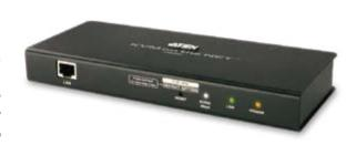
Because the CN8000 uses TCP/IP for its communications protocol, the server or KVM switch it is connected to can be accessed from any computer on the Net – whether that computer is located down the hall, down the street, or halfway around the world.
