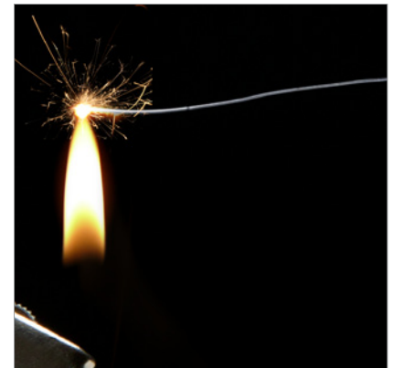
Figure 3: was processed in the wire CCS, the conductor glows and sprays sparks - similar a miracle candle (because of the CCS conductors the additionally added magnesium).
