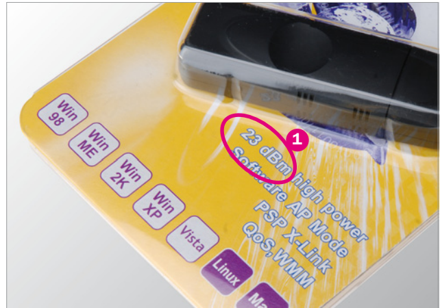
Fig. 2: 1 Already the packing betrays the unauthorized transmitting power. Maximal 100 mW, which correspondes to 20 dBm, would be permitted.
