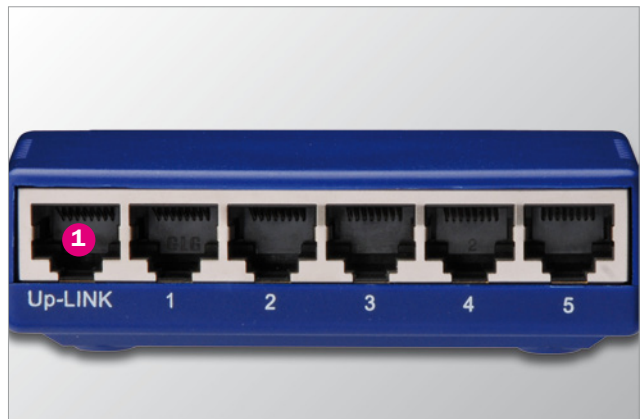
Fig. 4: 1 Like this Switch represented here, many network- products of the lower price segment do not contain an automatic medium recognition “Auto MDI (x)”.
