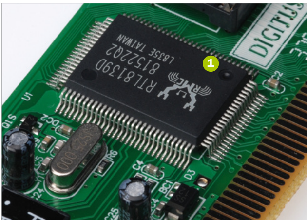
Fig.3: 1 Original Realtek type of network - chip on DIGITUS® network map - with users estimated for the extensive compatibility to usual market, in addition, also less spread operating systems.
