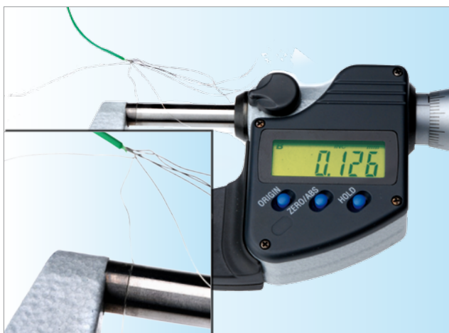
Figure 3 : In DIGITUS® cables excluding appropriate AWG- values (here 7 conductors 0.126mm = AWG 28) of the conductors are used, which guarantee an optimal function and life time.
