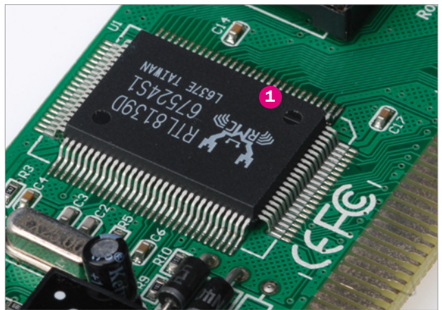
Fig. 4 : 1 This almost perfect falsification exclusively works with current Windows operating systems. Annoyance with the product is initiated, as soon as the user begins an operating system e.g. begins Linux, then the falsified chip refuses its service by system crashes.
