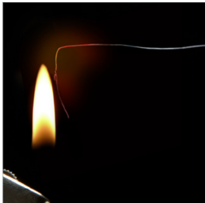
Figure 2: The conductor glows, breaks downward off and-evaporated. In this case it acts in all probability on CCA, thus the inferior copper / aluminum mixture.
