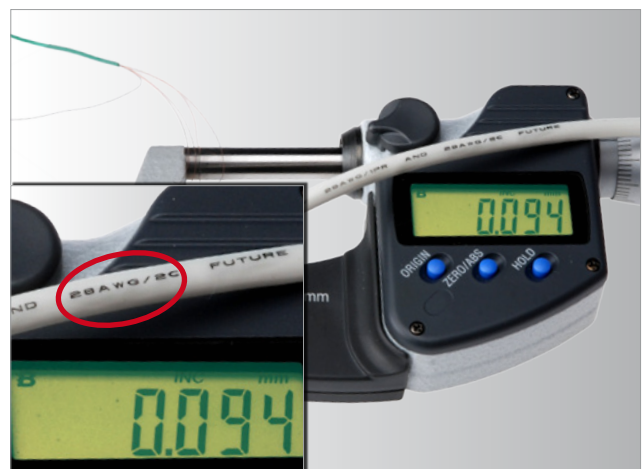
Figure 4: The cable is proven with the strand diameter "AWG 28" (=0.127 mm strand diameter) although a by far smaller diameter (0.094 mm = AWG 32) of the only 5 blocked strands is used.
