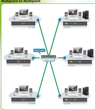
In multipoint configurations, the IGMP (Internet Group Management Protocol) function of your network switches/hubs should be enabled to avoid deterioration of data throughput. If you do not know how to enable IGMP, please contact your network administrator.
