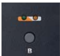
■ Power control buttons two function choices: Remote Access Enabled/Disabled; Power On/Off (Local Mode)
