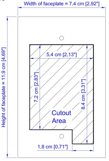
**Note:** ATEN recommends a 1-gang wall box with a depth of at least 5 cm (1.97 inches) to accommodate the connectors and cables.
