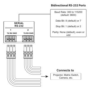
Connect to devices for controlling and receiving status messages from them. For bidirectional RS-232 control, the transmit (TX), receive (RX) and ground (GND) terminals must be wired on both the ATEN Control System and the device connecting
