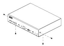
2. Using the 2 bottom screws from step 1 and 2 M3x6 screws from the rack mount kit, secure the mounting brackets to the sides of the VK1100.
