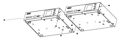
2. Use 4 of the screws from step 2 to secure the two VK1200 units together with the link bracket. Then install the left and right mounting brackets onto the sides of the units using 2 of the M3x5 and M3x6 screws included.
