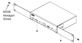
3. Use 4 self-supplied screw to secure the mounting brackets onto the rack.
