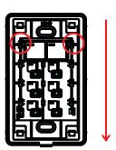
**Caution:** When removing button caps, place your fingers on the top of button caps and then press downwards, as illustrated below.
