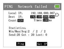
If the IP camera or network device is not configured properly or not plugged in, it will say "network failed", send and received package number is 0, have 100% packet loss. If the tester connects to the device, it will say "network succeeded", send and received package number are the same, have a 0% packet loss.
