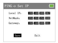
Application: PING testing is the most conventional network debugging tools. It is used for testing if the connected
