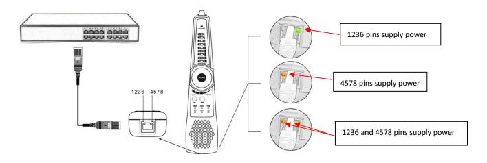
**Application:** Checking the pins used of PoE switch or other device for power supply, to avoid cause cannot supply power or camera and other device damaged. Can detect the voltage of POE power supply device, PoE is standard or non-standard.
