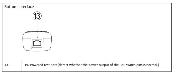
Note: Receiver port continuity detection only supports the local end, does not support the remote end. Emitter can support the near end, middle end and far end port detection.
