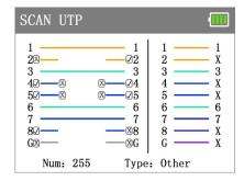
As shown above, the right side of interface is the continuity result of cable tester and wire receiver ports, the left side is cable's sequence.
