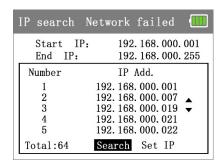
Press key to "Set IP" function, press to set the tester's IP address, the tester's IP address must be same network segment with the scanned network equipment, and select the "Scan" and press confirm key, then can guickly search the IP address of the IP camera or other equipment connected to the tester.
