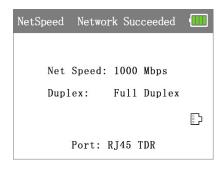
Connected to the tested IP camera or Ethernet device to tester, the top of the screen shows "network succeeded", can automatically detect and identify information such as connection speed and duplex mode. If it says "network failed", please check whether the connection port is correct and whether the connected device is working normally.
