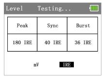
Press key to switch the MV and IRE (Institute of Radio Engineers) mode, NTSC format uses IRE as the unit of measurement, and PAL format uses mV as the unit of measurement.
