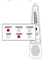
The 1-8 indicators on the cable tracer will flash in sequence according to the network cable sequence, will display the cable type through the "Direct/Cross/other" indicator.
