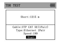
If want to test "UTP CAT 5E (4 pair) or UTP CAT 6E (Pair)", please connect the cable to "TDR 2.0" port.
