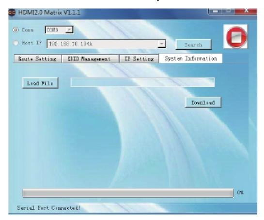
At System Information you can Upgrade the Firmware of Matrix Switch NOTE: The Firmware File need to be supplied by the manufacturer
