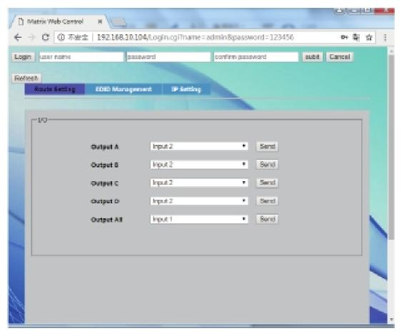
At the Route Setting interface, you can set any input port to any output port one by one, or anyone input port to all output port.
