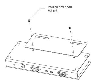
2. Screw the bracket into any convenient location on the rack.
