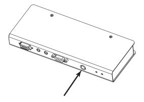
**Note:** Remote mode cannot be selected. The remote console can get control only when the Operating Mode Pushbutton on the CE750AL is toggled to *Auto* and the local console is idle. If the remote console is then idle for more than five seconds, the local console can gain access.
