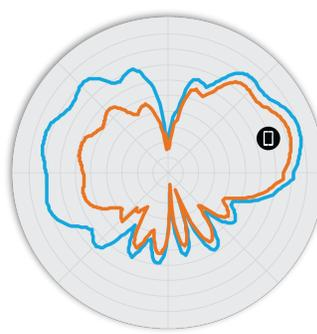
Figure 5. R730 5GHz ElevationAntenna Patterns
