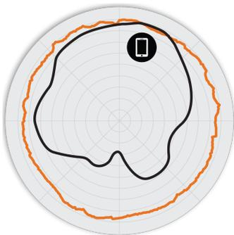
Figure 3. R730 5GHz AzimuthAntenna Patterns
