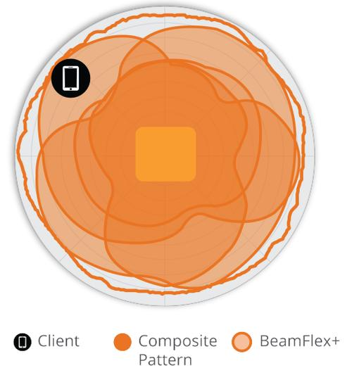
Figure 2. R730 2.4GHz AzimuthAntenna Patterns
