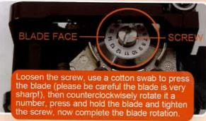
You need to cleave the fiber and check if the cleaving face meets the requirements, if it works well, you do not need other operations.
