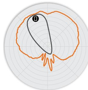
Figure 5. M510 5GHz Elevation Antenna Patterns
