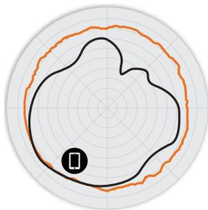
Figure 3. M510 5GHz Azimuth Antenna Patterns
