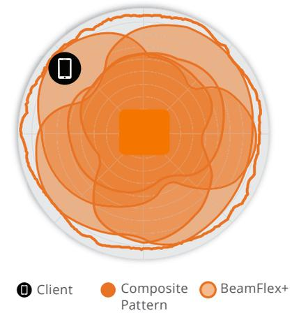
Figure 2. M510 2.4GHz Azimuth Antenna Patterns
