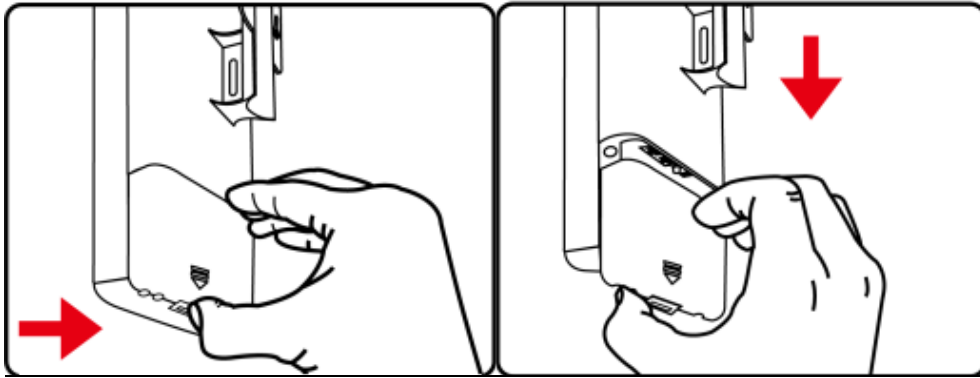
Figure 3-1 Connect the Antenna
