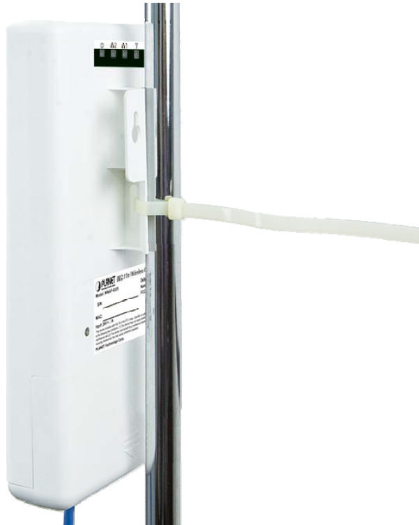
Figure 3-6 WNAP-7325 Pole Mounting
