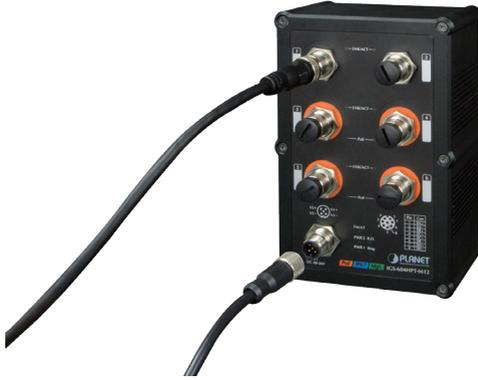
**Step 5:** Turn clockwise to tighten the screw nut of the M12 power connector.
