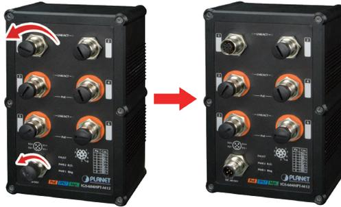
**Step 2:** Insert the M12 UTP male connector into the M12 female Gigabit Ethernet port of the Industrial Managed Switch.
