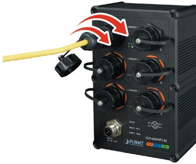
**Step 4:** Insert the waterproof M12 power connector into the port of the power input.
