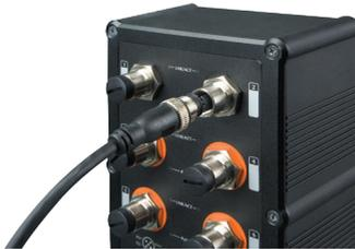
**Step 3:** Turn clockwise to tighten the screw nut of the M12 connector and make sure the connection is tight.
