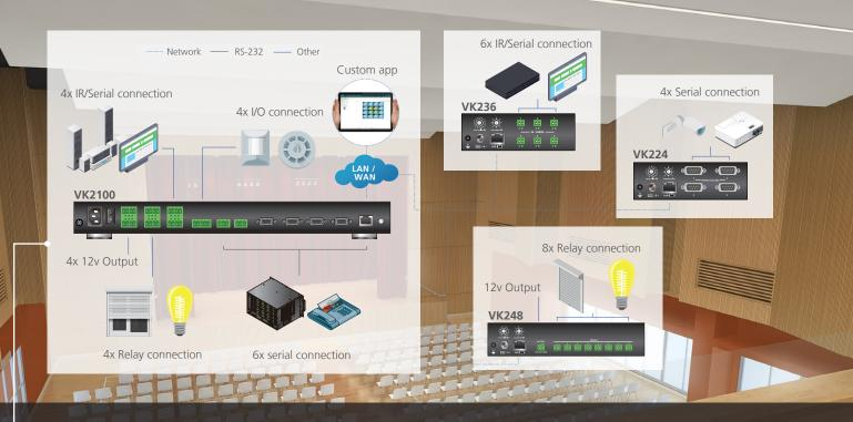
The ATEN Control System can easily be deployed into an existing installation - in a variety of commercial and educational environments, as it seamlessly integrates with a wide range of hardware devices, including A/V equipment, video matrix switches, cameras, power supplies, conference systems, projector lifts and many more. The ATEN Control System is perfect for meeting rooms, conference centers, boardrooms, classrooms or any room that requires complete control of all hardware equipment.
