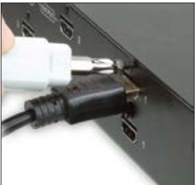
1 Loosen the screw above the port
