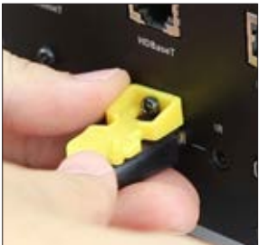
2 Slide the LockPro™ over the loosened screw
