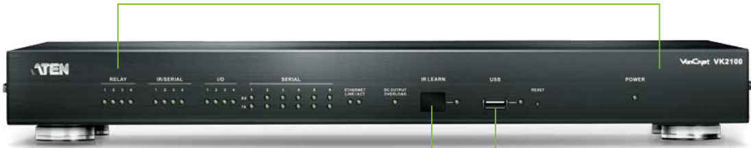
LED indication for hardware status and active messages
