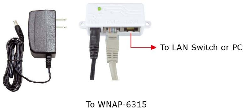
Figure 3-3 Connect the PoE injector
