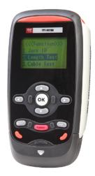
TPT-8020A is an easy-to-use and portable test set with advanced cable locator and simple network tester in one unit. Besides identifying wiremap, measuring the cable length, diagnosing cable faults and tracing cables, the TPT-8020A can also be used to simply perform network testing. It is an absolutely necessary tool for cabling construction and network maintenance.
